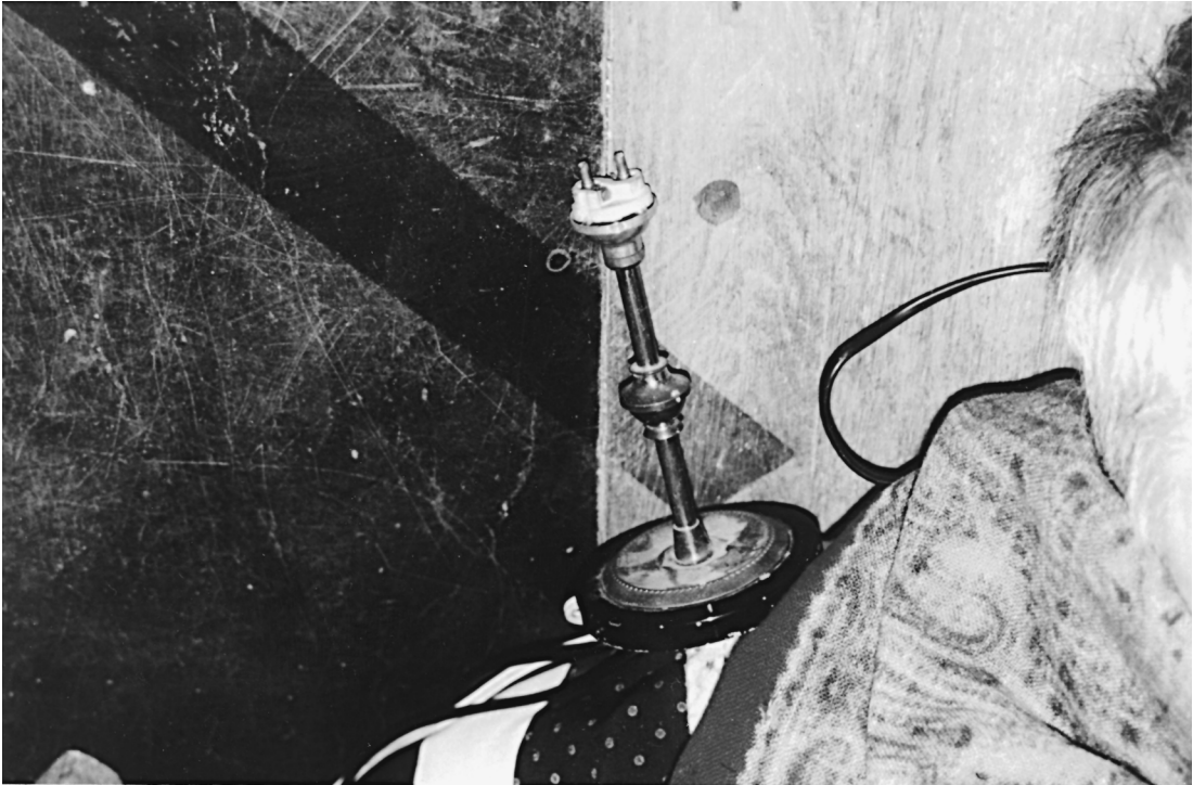
FIG. 1—Part of the body of the old woman lying on the floor and bedside lamp two metallic edges for electric contact left bare near her face.
